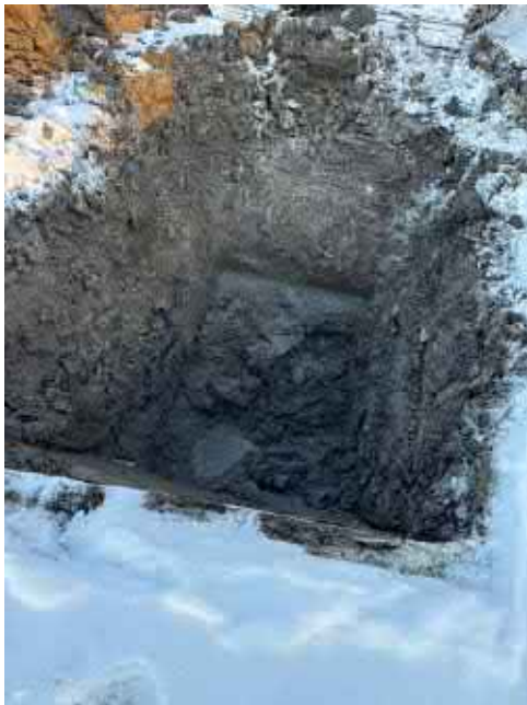
3.2m There was water at the bottom of the test pit.
